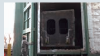
A large-capacity annealing furnace for relieving residual stresses and strains
