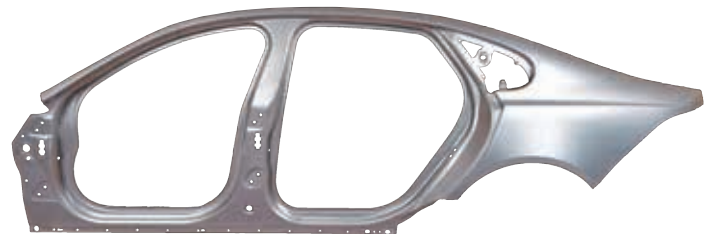
An aluminum vehicle side panel formed by an AIDA press
