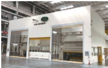
Large servo tandem line with a destack feeder unique to AIDA, installed at a joint venture manufacturing plant of a major British-Chinese automobile manufacturer
