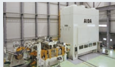
PMX-L2-16000 press capable of working with large dies and processing higher tensile strength steel parts for automobiles
