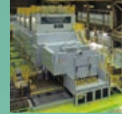
World's fastest servo press line (at the time of introduction) for automobile body panels
