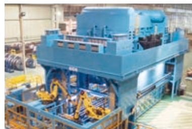
Servo transfer press for forming high tensile strength steel
