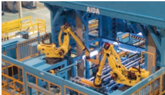
A destack feeder—an automated high-speed feeder that continuously supplies blanks one by one to a press
