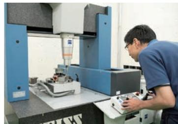
Using a three-dimensional measuring device
