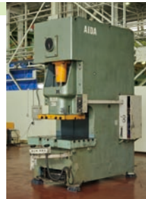
Retrofit example (converting a Mechanical Press to a Servo Press)
