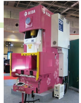
Retrofit example (converting a Mechanical Press to a Servo Press)
