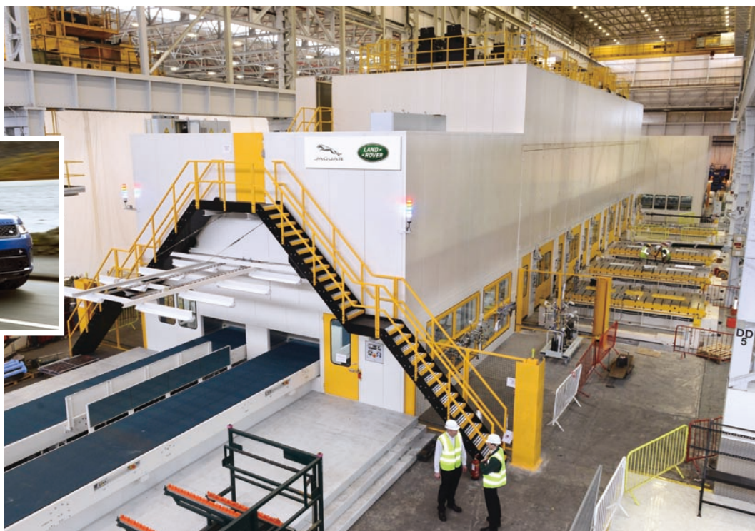
A large servo press line for forming automotive body panels
