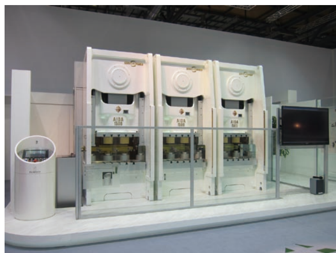
A line composed of multiple 150-ton press machines. With the 3 press machines lined up side-by-side it can also be utilized as a 450-ton press machine.
