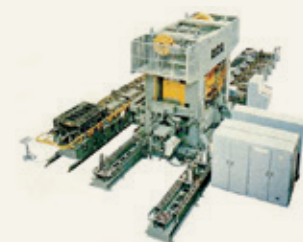
Mark IV Stamping Center System (3-D transfer)
