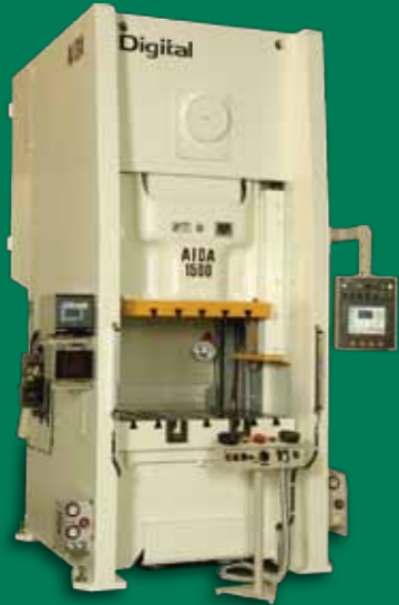
Digital servo former series NS-1-1500(D) World first direct drive servo press (2002, present direct servo former)
